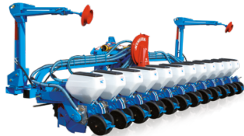
Semoir NC Technic Maïs 12 rangs repliable Double-barre (45cm)
